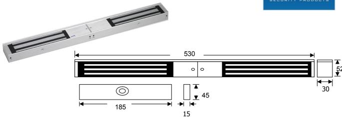
The EM08 double midi electromagnetic lock is a fail-safe design with no mechanical bolt and depending on the powerful magnetic force to secure and release the door are suitable foe use in areas which require security controlled access or egress such as exit door.
