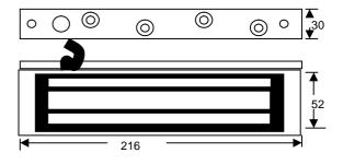
The EM06 magnetic lock is totally sealed in an epoxy sealed stainless steel case for water-resistant and vandal-resistant purpose. Offering up to 800lb holding force. It can be applied with access control. PLEASE NOTE: Holding force is dependent on door construction
