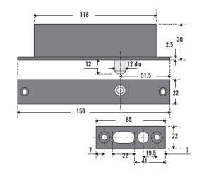
The compact size of this solenoid bolt makes it ideal for installations where space is limited and light usage is expected. It offers door position monitoring and variable re-locking delay.
