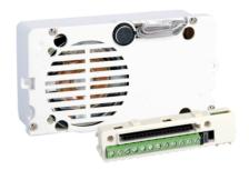
ViP system audio unit with facility for connection of a remote camera with 12Vdc power supply. Complete with terminal block and digital audio management system with Echo-cancelling, watertight loudspeaker and electret microphone, loudspeaker volume adjustable from the front. Dimensions: 102x55x38 mm. Compatible with H.264 video format.
