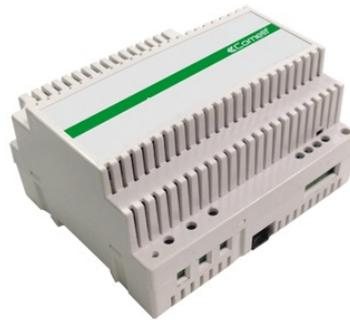
Power supply unit with 110-230 VAC primary and 33 VDC / 1.8A continuous output for 316 range entrance panels. Equipped with internal protection against current overload and short circuits. Dimensions: 106x89x62 mm (6 DIN modules). PSE certified.
