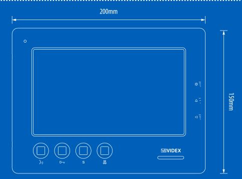
The 6700 series surface mount video monitor with a 7" Hi-Res full colour active matrix LCD screen is designed primarily for low and high-rise private developments and individual houses where an attractive and cost-effective functional videophone is desirable.
