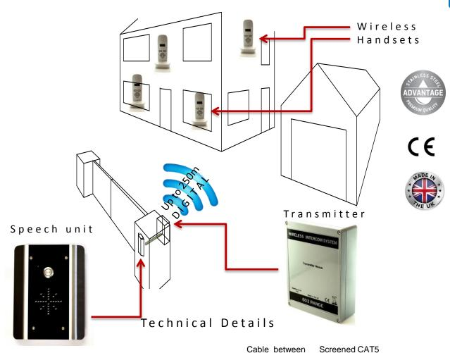
speech unit & transmitter Power Supply 12v dc (adaptor included) Max cable length 8 meters (recommend short as possible) **Current Consumption** 50mA standby, 250mA calling Cable cores 2 x SPK, 2 x MIC, 2 x power, 2 x **Relay Outputs** button N/O & N/C contacts Relay type Speech unit IP rating IP55 Relay time Fixed 4 seconds Transmitter IP rating IP65 Relay load 2A 24v AC max Manufacturer 2 year return to base warranty Technology type 1.88GHz DECT Digital Warranty
